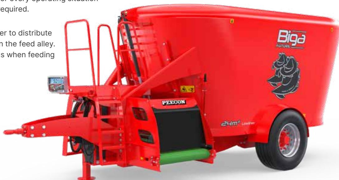
Unloading doors are optionally available with a height-adjustable conveyor belt. Some models are also available with a chain conveyor instead of a conveyor belt.
