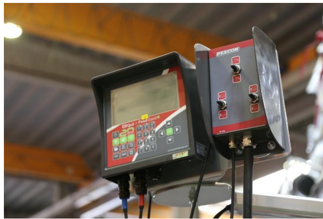
Figure 7-2 Peecon control panel i.FeedGood weighing computer (left)
