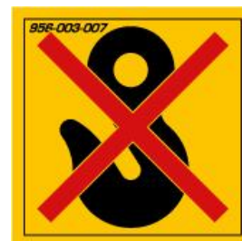
Figure 5-3 Unsuitable lifting point
