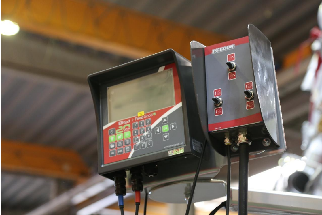
Figure 7-2 Peecon control interface i.FeedGood weighing computer (left)
