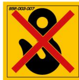
Figure 5-3 Unsuitable lifting point
