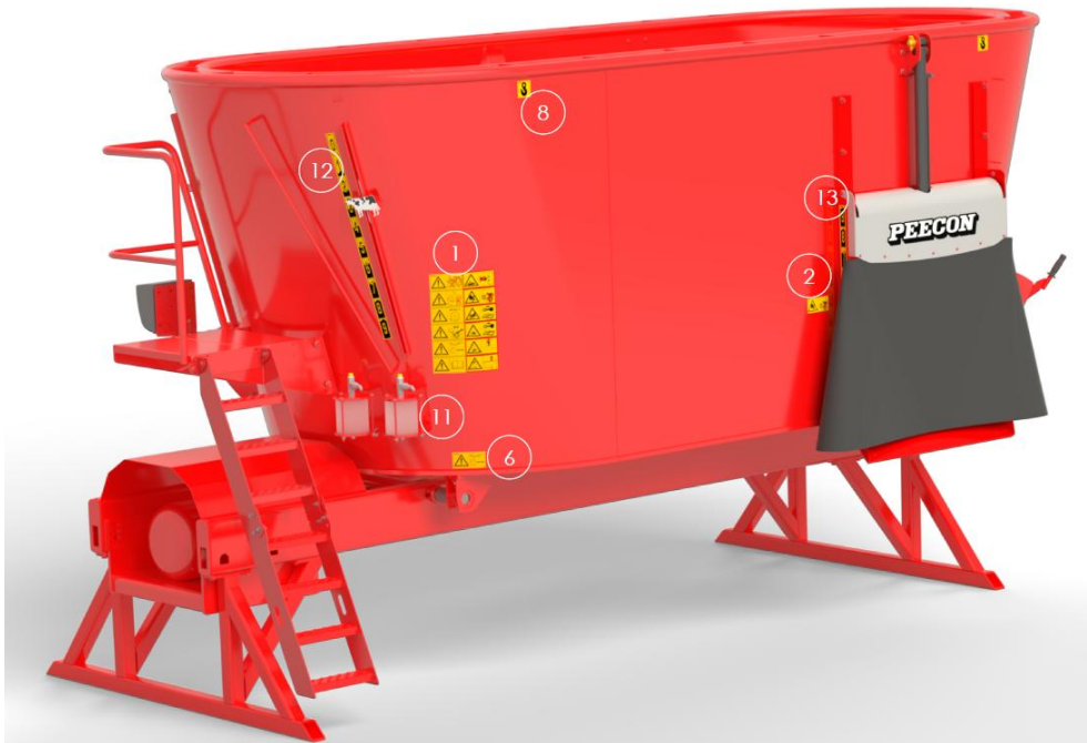
Figure 5-6 Safety symbols on a Biga stationary cut mix tub
