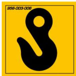
Figure 5-2 suitable lifting point
