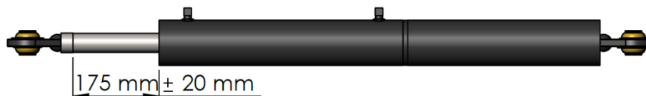
Figure 13-1 Extension length of the command cylinder in the neutral steering position
