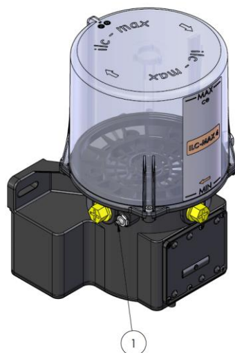
Figure 6-2 Lubrication system refill grease nipple
